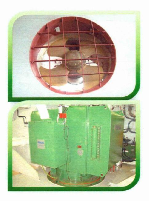
Each propeller is 8' in diameter, weighs 6.6 tonnes and has 1.8 MW of power i.e. 2,450 H.P, about 20 full sized family cars.
